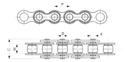
$\begin{array}{lll} \text{Breaking power} = 172400 \\ \text{C} & = 54,40 \\ \text{Chain size} & = 1"3/4 \\ \text{d} & = 12,70 \\ \text{D} & = 25,40 \\ \text{Description} & = 140 \\ \text{P} & = 44,450 \\ \text{W} & = 25,22 \\ \end{array}$
